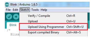
The LED2 on the AVR USBASP Programmer board will ON during the uploading process. After done uploading, there will be SCK warnings appeared at the bottom of the Arduino software. These warnings can be ignored due to the firmware version of AVR USBASP Programmer. It does not affect the result.
